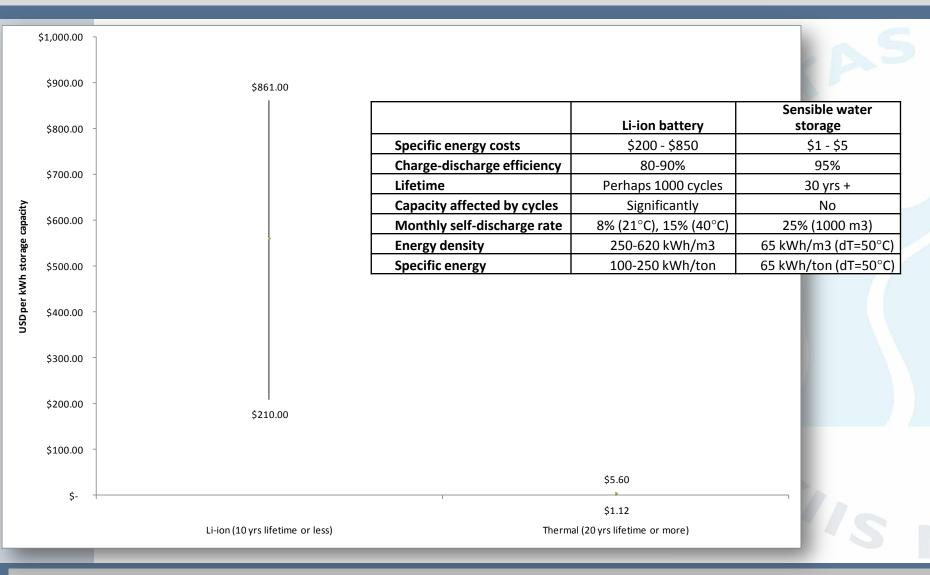
Specific investment costs (USD/kWh) for li-on battery data versus sensible water thermal storage. Li-on data: Delucchi, M.A., Jacobson, M.Z., 2011. Thermal storage data: Author.
